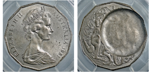
38 1981. Obstructed strike; indented with a 2 Cent sized (21mm round) blank planchet to right of Reverse leaving a large depressed impression. PCGS graded MS 63 (81763009). The only example of this major error type we have seen, and probably unique. Ex IAG SVS 1 October 216 (Lot 516). Ch.UNC
