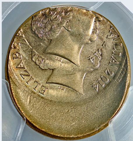
54 2014 Anzac Centenary. Struck twice off-center; once 25% and once 60% causing a large spread flan with a slightly raised large off center rim lip. PCGS graded MS 65 (37155128). A stunning error in beautiful condition and extremely rare, with no other graded examples. GEM UNC
