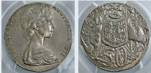
37 1976. Struck on a 20 Cent planchet. PCGS graded MS 64 (37155123). Slightly off-centre with part edge design and lettering missing from the smaller planchet. Light old tone. A very rare and possibly unique error for this year. Ch.UNC/GEM
